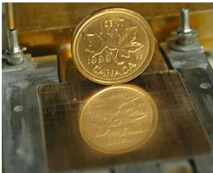
You can see a few insignificant scratches on the copper, which I noticed after taking the picture, so of course I went back to sanding ;) If I do this again in the future I will try to get a grit higher than 1200, since I couldn't remove all the scratches. No matter how much I sanded, I ended up with the same results. So I finally settled
