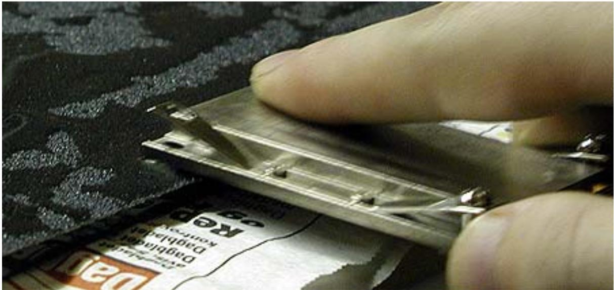
The next picture shows most of the raised surfaces removed except for one which is circled once again in red. I hadn't realized it was there until I took the picture, so back to sanding...
