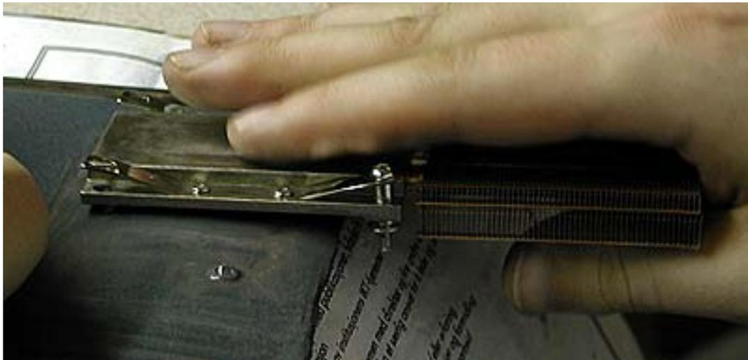
You can see from the bubble in the picture that I am keeping the paper wet. There is a mirror underneath to keep the sandpaper as flat as possible, but any flat glass surface can be used.
