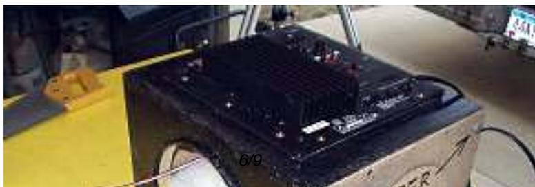
Next, install the speaker, making sure to get the wiring polarity correct and using the same #6 x 3/4" panhead screws to install the speaker. Finally, install the grille - I used some finish nails as I mentioned above and used a black magic marker to touch up the nail heads. They will be virtually invisible from more than three feet away. Here's a look at the final subwoofer on the bench.
