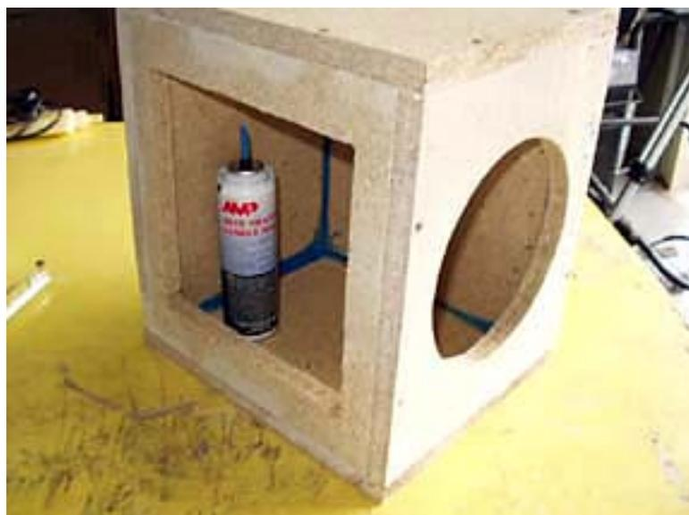
After the glue is dry, the screws are in place, and the box assembly is complete, it is time to make a frame for the grille. I used some 3/4" pine scraps ripped to appx 1/2" wide. Once again, use a bit of glue and a couple of 4d finish nails. Use a small piece of medium or fine sandpaper to round off any rough edges. Additionally, it would be a good idea to pre-fit the subwoofer and make sure the grille frame will fit correctly. Because I
