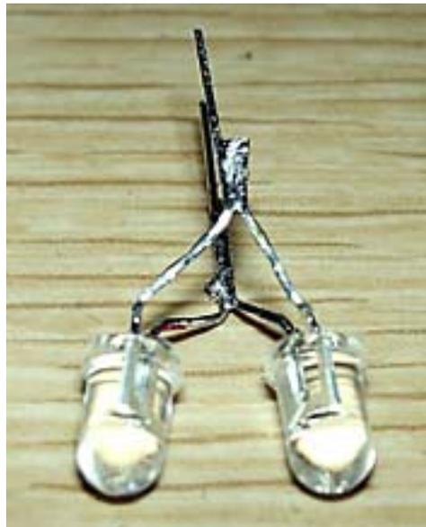
Remember that the area where the legs of the LED's are welded will not fit into the audio header we are using for a power lead so I kept the area welded to 3mm to prevent too much "outhead". Now plug that sucker into the sound cable like this:
