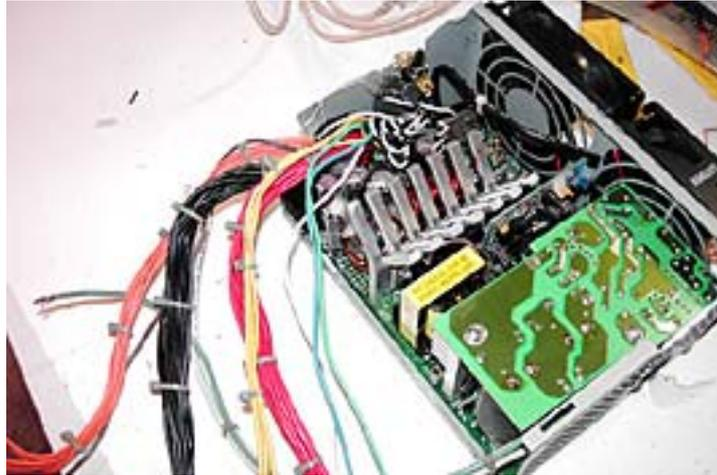
Next, I removed the power input plug. I did this carefully, because I planned to use it elsewhere in the box. I pulled out the internal AC feed wires and spliced in a longer length of heavy duty wire to give me some room to work with.
