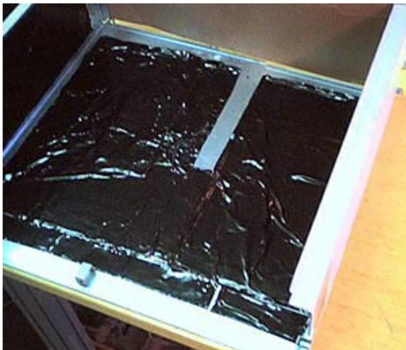
Removal was MUCH easier. Obviously, the manufacturer of this product has given the foil a better bonding agent than the adhesive on the application side. The strength of the foil prevented the product tearing that occurred with the AMT045/VBV-2HD, so removal took only moments and was far easier to accomplish. It seemed like the application adhesive left far less residue, in fact, it all came off. That's a definite plus in my book.
