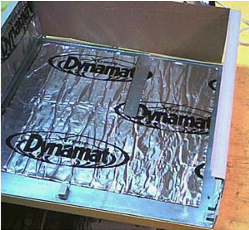
The installation was straightforward and removed exactly like the Accumat VB-2MAX. Note the logo in the picture above... if you have any windows cut in the side of your case, this will be noticeable. This product might bring a huge plus to the table if you have any cathode or led lights installed inside your case, as it will be very reflective and should make your case seem much brighter.
